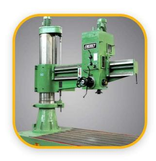
A drill head is mounted on the radial arm, allowing it to move along the arm and position the drill spindle precisely over the workpiece.
